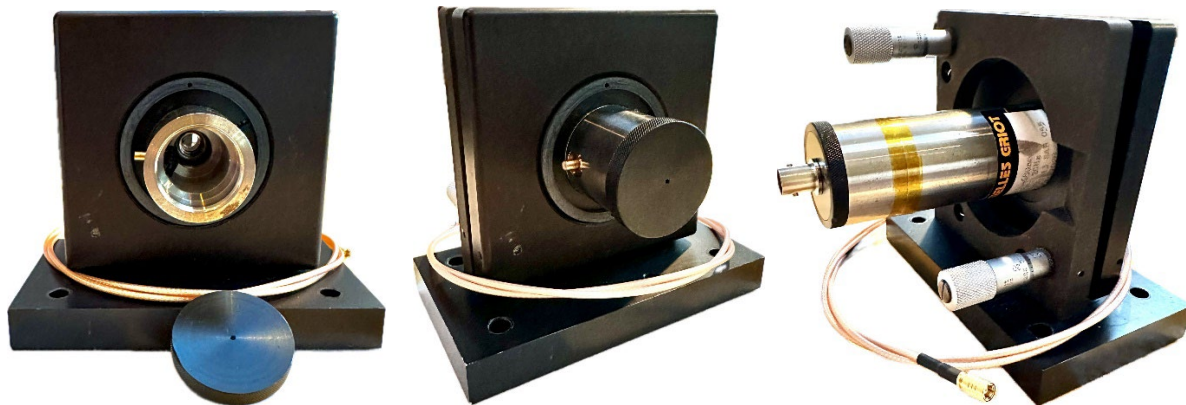
Figure 4 SFPI head, front with cap off, front with cap on, rear view.
