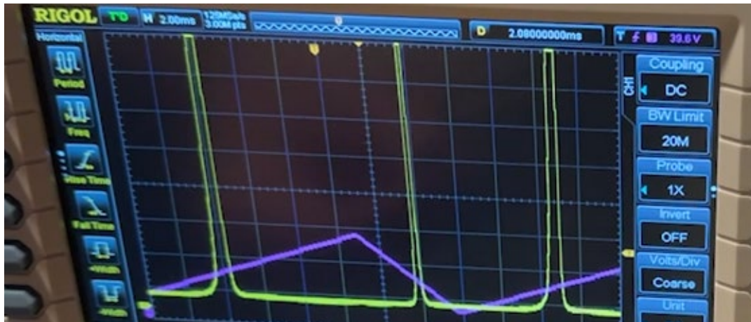
Figure 17 MG OSA SCAN Range knob after being rotated CCW for a single SFPI head sweep.
